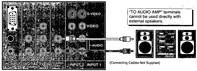
Adjustment - When an audio amp is connected to "TO AUDIO AMP" terminals:
